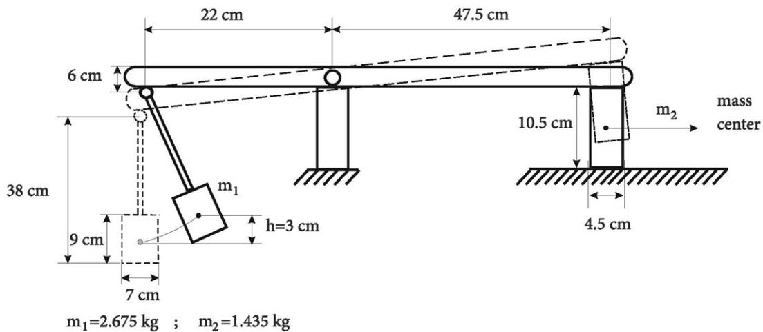
When I lifted the pendulum mass center (weight with mass  $m_1$ ) to 3 cm, as shown above, the pendulum started to swing and centrifugal force, influencing the lever by the pendulum, started to lift the weight with mass  $m_2$  on the other end of the lever. Lifting of the weight on the other side of the lever was periodical and at different heights.
